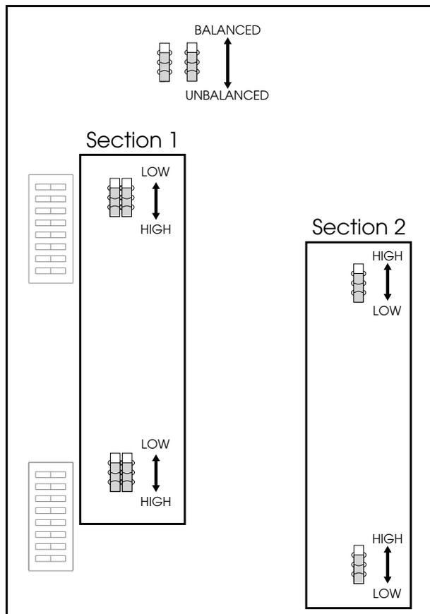
2. In order to set the input loading you must toggle the DIP switches which are located on the main board of the preamplifier. Each one of these switches connects a resistor or capacitor in parallel with the input and so adjusts the load value. The default values are 47kΩ and 50pF. Refer to the diagram below, which is repeated inside the unit, to determine the values which need to be switched in for your cartridge. Replace the cover after setting the switches.
